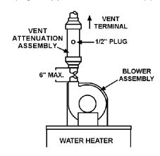
FIGURE 22: Typical Vertical Installation
